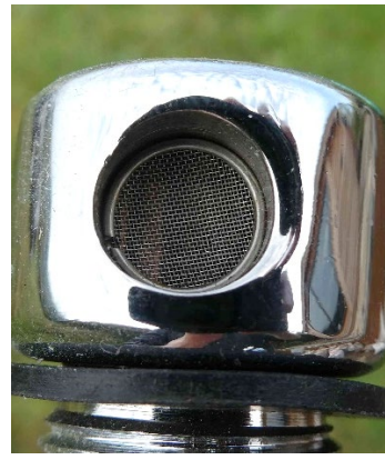
Proprietary flame arrest with a mesh of greater than 11 wires/cm
