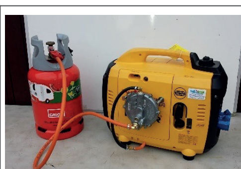
A LPG-powered portable generator/invertor
